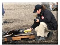
Deputy Fire Marshal Jess Sinerius, using the PID to monitor for the presence of ignitable liquid vapors
